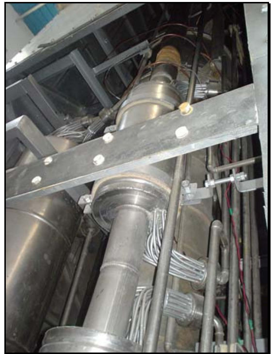
Argon welded leakproof stainless steel columns, with all stainless steel lines.
